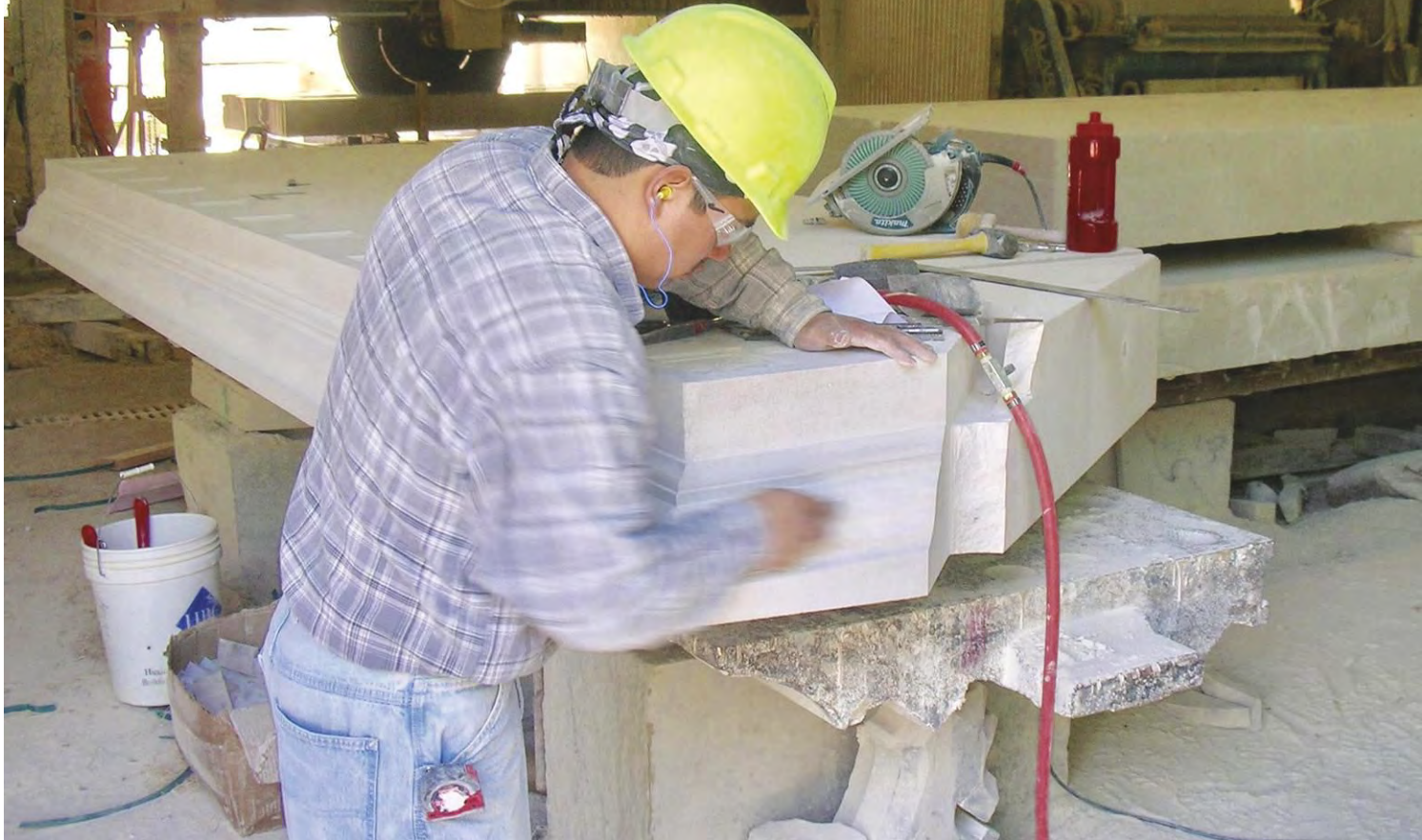
The Indiana limestone pieces were all cut on their natural bed (horizontal grain) at Galloy & Van Etten, Inc.'s fabrication shop.
